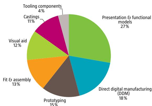
**Figure 2: Uses of Direct Digital Manufacturing**
